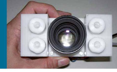
The mechanical assembly of these components into a common housing has been designed to be in line with the requirements of the mounting restrictions of the front nose of the flight robot. Figure 1 shows the Time of Flight camera mounted in the front part of the flight robot directly looking at the observed image scene.
